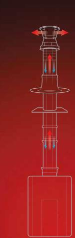
Venting available in vertical and horizontal configurations. Concentric structure allows hot exhaust to exit through interior tube, while fresh air enters through the outer layer.
