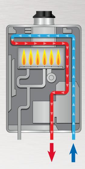
The tankless burner is on only when hot water is needed
